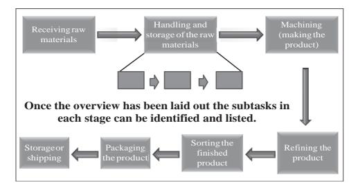
FIGURE 10-1: Overview of a seven-stage manufacturing process © 2008 Jonathan T. Scott
