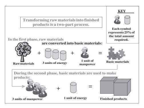
FIGURE 5-1: Stahel's ratio for manpower and energy use in production © 2008 Jonathan T. Scott
