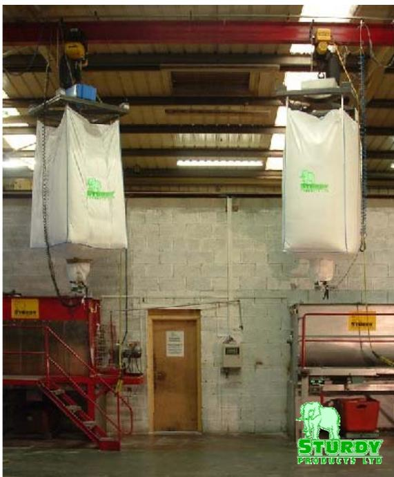
Photo 2 The new bulk handling system and mixing tank
